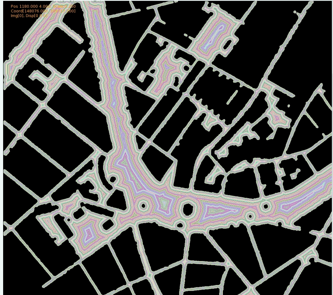
Distance transfo and gap filling
